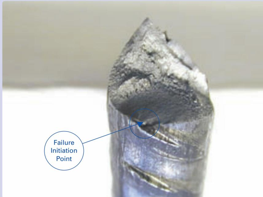
Figure 3 Failure initiated at base of transverse rib
